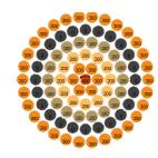
Centro-symmetrical layout is ideal to generate Zernike polynomials in closed-loop and open-loop
